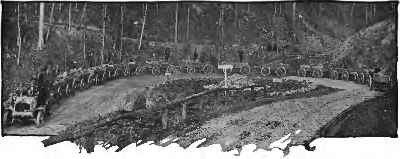
Packard truck of 3 tons capacity drawing a wagon train of fifteen wagons up a North Carolina mountain
